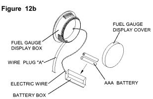
IMPORTANT: When the gas tank is removed from the tank pull-out tray, the fuel gauge display will not operate.
